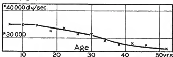
FIG. 7.—Dependence of highest audible tone upon age of subject ( 44 ). * It is probable that these frequencies should be divided by two.
